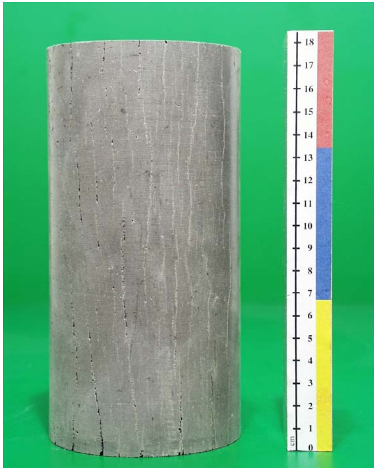
Plastic bag sealed and stored claystone sample (6 weeks storage time)
