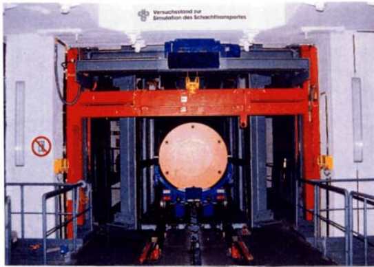
Hoisting Cage for 85t Payload
