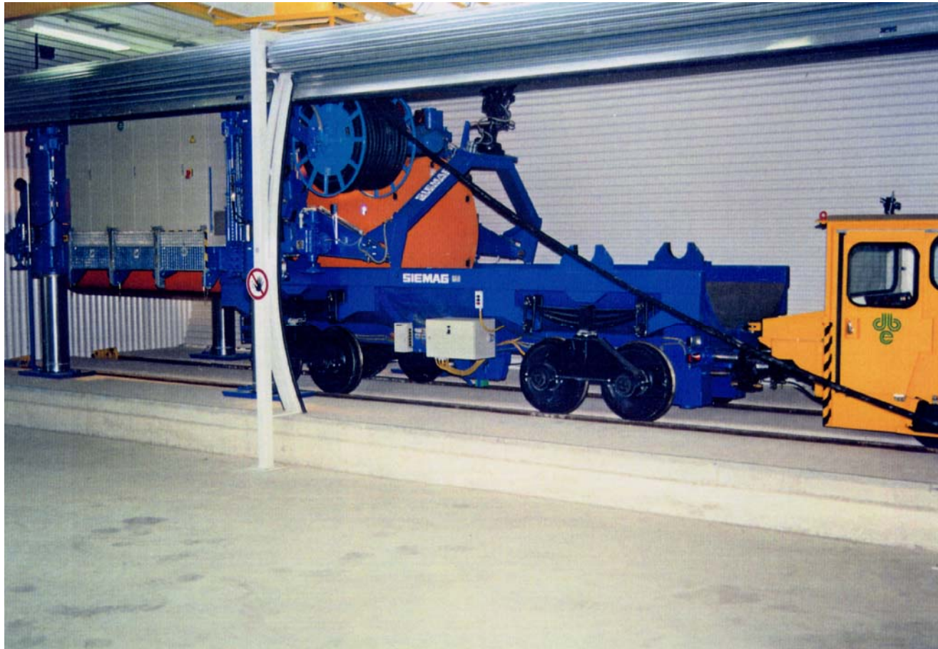
Full-scale demonstration of the POLLUX emplacement system at the test site in Peine
