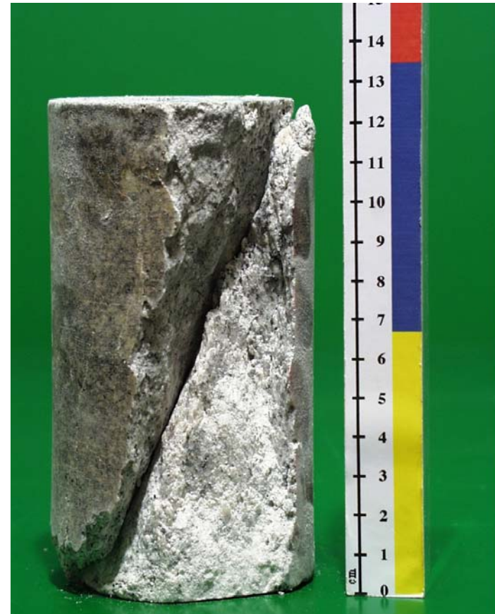
Test sample before and after failure with single macro-fracture (different scale)
