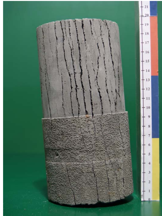
Ageing cracks in plastic bag sealed and stored claystone sample (6 months storage time)
